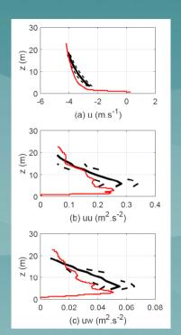
Comparison of the Reynolds stresses derived from ADCP measurements and simulation data.
