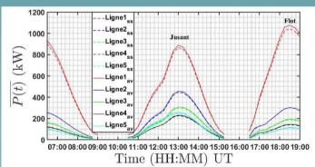
Blockage effect in Actuator Disk tidal turbine modelling (Dirieh et al., JH2020). Right: velocity difference with and without blockage effet in a tidal farm in the Raz Blanchard. Left: Tidal farm power with blockage effet (---) and without (\_\_\_\_).
