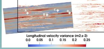
Average longitudinal velocity and velocity variance at a 15 m depth for flood (iso-surfaces) and ebb (iso-contours).
