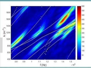
Enable to detect on which side the delamination is (here on the composite side)
