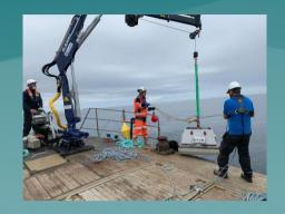
Recovery of the first samples (coupons) and deployment of the new ones to be performed in Sept/Oct. 2021.
