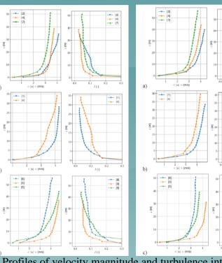
Profiles of velocity magnitude and turbulence intensity at Flood (Left) and ebb (Right) peak at several locations
