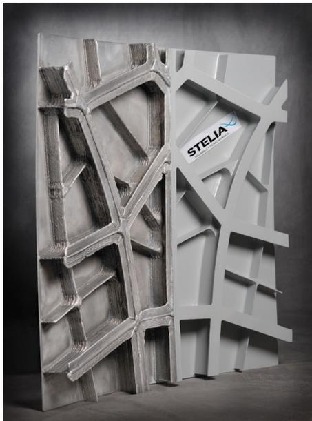
**The 3D printed fuselage panel - the rough printed surface on the left, the polished and painted surface on the right**
