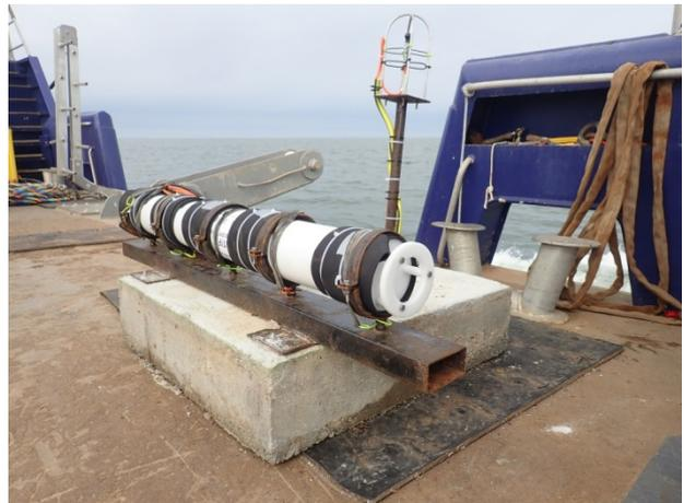
*OSEAN recorder installed on SEM-REV*
