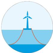
**A world first in anchoring.** Floatgen's semi-slack anchoring system (to keep the turbine in the correct position) is innovative in its use of synthetic fibres (nylon) as opposed to chains. A world first for permanent anchoring at this scale (6 anchoring lines).
