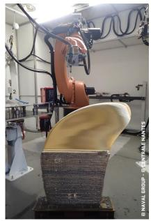
Vincent Geiger, Director of Naval Group's Naval Research Technology Research Center, stressed the significance of these initial results: "Printing this demonstrator is a major step towards the manufacture of innovative propellers by additive manufacturing. These initial results mean that it's possible to envisage the short-term commissioning of differentiated propellers for the ships that will use them."
