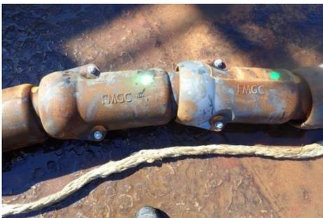
The FMGC shells protect, stabilize and restrict the bend of subsea electrical cables. The objective of the tests is to demonstrate the stability of the cables ballasted with these cast iron shells, including under heavy swell conditions. The shells will remain on site for several months and will be subjected to extreme winter conditions. These tests will
